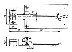
The thermostat has a normally open contact which closes at a typical plate temperature of 35  $\pm3$   $^{o}C$  and reopens at 30  $\pm3$   $^{o}C$
