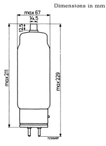
Mounting position: Arbitrary between horizontal and vertical with base down
