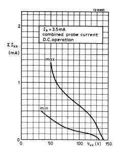
COMBINED PROBE CURRENT TO ALL NON-CONDUCTING CATHODES Sum of the probe currents to the non-conducting cathodes (  $I_{kk}$ ) plotted against the voltage difference between the non-conducting cathodes and the conducting cathode (V $_{kk}$ ), showing the minimum and maximum values of probe current for a particular cathode current ( $I_k$ ).
