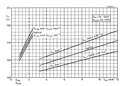
$<sup>^1)</sup>$  The decimal point maintaining voltage  $V_{\mbox{mdp}}$  and the punctuation mark maintaining voltage  $V_{\mbox{mpm}}$  include the voltage drop at the 10 k $\!\Omega$  series resistor.
