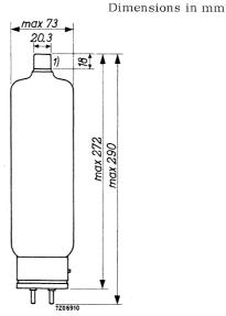
$<sup>^{1}</sup>$ ) Cross section of flexible anode lead at least 10 mm $^{2}$ .
