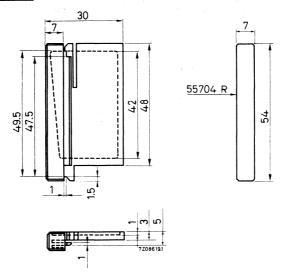
These two items are supplied together under type number 55704 Snap-fit tube holder Type number 55703
