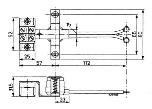
The thermostat has a normally closed contact which opens at a typical plate temperature of 52  $\pm3$   $^{O}C$  and recloses at 41  $\pm3$   $^{O}C$
