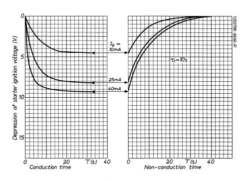
Formation and recovery curves of the starter ignition voltage for a nominal tube
