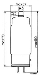
Mounting position: Arbitrary between horizontal and vertical with base down
