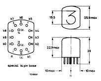
1) Centre line through pins 6 and 12 (Note: distance between centre lines of adjacent tubes must be at least 20 mm)
