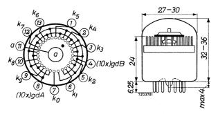
$K_0$  is aligned with pin 7 to within  $\pm 3^{\circ}$
