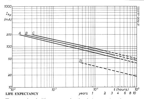
The curves show the life expectancy when the tube is run continuously at room temperature.
