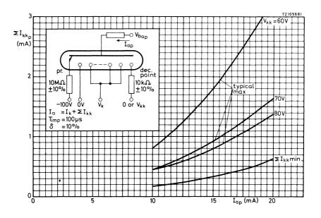
Long life cold-cathode ten-digit indicator tube for side-viewing.
