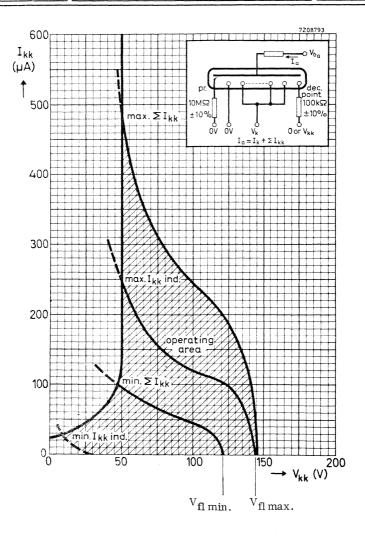
$I_{kk}$  individual and  $\Sigma I_{kk}$  versus cathode selecting voltage  $V_{kk}$  at  $I_a$  = 2.5 mA.  $I_{kk}$  and  $\Sigma I_{kk}$  are proportional to the anode current within the operating range of  $I_a$  and with  $V_{kk}$  = 0 V to 100 V.
