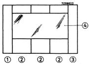
The various items can be fitted easily into a rectangular window cut in the frontplate of a piece of equipment; no tools are needed for mounting and this can take place from the front.
