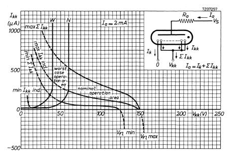
For low cathode selecting voltages the current  $I_{kk}$  to the "off" cathodes will increase and the readability of the "on" cathode will be affected. It is therefore recommended to use a nominal operating point to the right of line N. Under the worst operating conditions the operating point should never reach the area left of line W.
