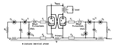
Capacitor value C 2 8  $\mu F$  Capacitor voltage V<sub>C</sub> 650 400 V  $\pm$  10% Peak value of closed circuit current 80 to 100 A
