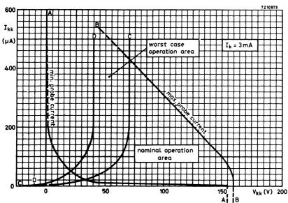
PROBE CURRENTS TO INDIVIDUAL NON-CONDUCTING CATHODES
