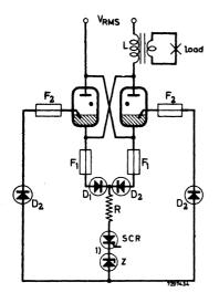
$V_{RMS}$  220 250 380 500 600 V R 2 2 4 5 6 Ω  $F_1$  = 2 A fast response time  $F_2$  = 10 A fast response time Z = zener voltage ≥ 18 V
