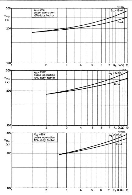
PEAK SUPPLY VOLTAGE AS A FUNCTION OF ANODE LOAD RESISTOR
