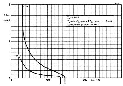
COMBINED PROBE CURRENT TO ALL NON-CONDUCTING CATHODES
