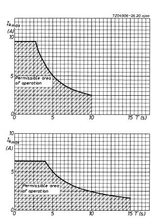
The top curve shows the maximum number of seconds in any 10 second period for which a given average current may be drawn from a sinusoidal supply if the peak voltage applied to the tube is less than  $1.25~\rm kV$ . The bottom curve shows the maximum number of seconds in any  $15~\rm second$  period for which a given average current may be drawn from a sinusoidal supply if the applied peak voltage lies between  $1.25~\rm and~1.5~\rm kV$ .
