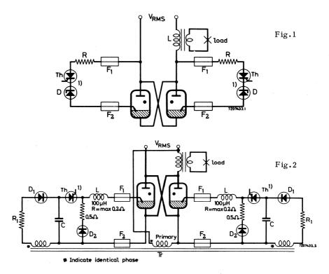
The ignitor must be connected to its control circuit by a screened lead which affords protection against R.F. fields. It is inadvisable to operate separate excitation in the absence of anode mains voltage.
