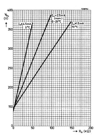
Graph denoting the relationships of D.C. anode supply voltage and required anode resistor to remain within the recommended operating region.
