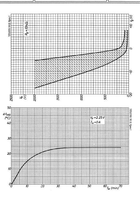
Thyratron, inert gas-filled triode for power control and ignitor firing.
