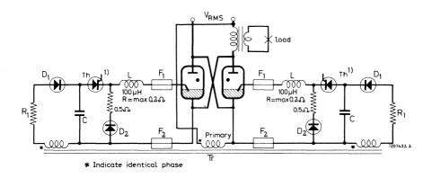
Capacitor value 2  $\mu F$  Capacitor voltage 650 V  $\pm 10\%$  Peak value of closed circuit current 80 to 100 A
