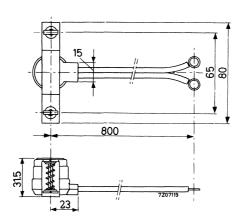
The thermostat has a normally closed contact which opens at a typical plate temperature of 52  $\pm 3$  °C and recloses at 41  $\pm 3$  °C
