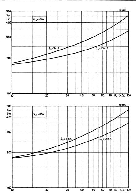
D.C. SUPPLY VOLTAGE AS A FUNCTION OF ANODE LOAD RESISTOR
