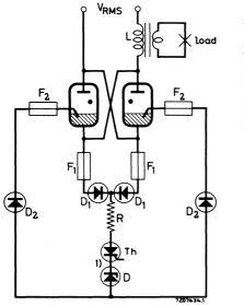
$V_{RMS}$ 2  $\Omega$ 2 A fast response time  $F_2 =$ 10 A fast response time D zener voltage ≥ 18 V
