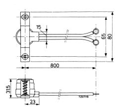
The thermostat has a normally open contact which closes at a typical plate temperature of 35  $\pm$  3  $^oC$  and reopens at 30  $\pm3$   $^oC$
