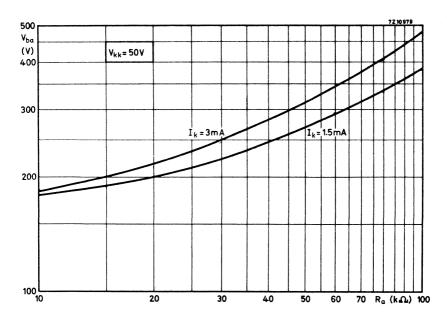
D.C. SUPPLY VOLTAGE AS A FUNCTION OF ANODE LOAD RESISTOR NOTE - The supply voltage/load resistor curves are derived from:
